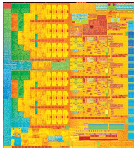
The Intel Xeon E3-1200 V4 die. The chipmaker has started integrating Iris Pro graphics into the same chip. Image courtesy of Intel.
