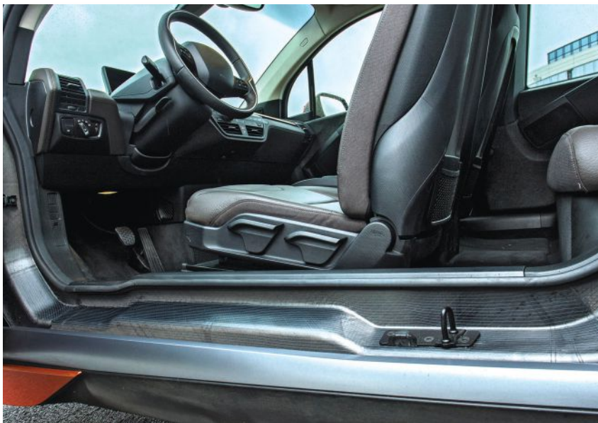
The use of industrial adhesives allows automakers to explore bonding options that involve less welding and bolting, thus reducing the vehicle's noise, vibration, and static and dynamic stiffness. Image courtesy of Dow Automotive.
