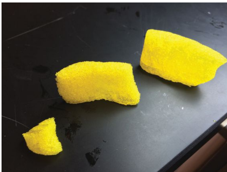
Printed on Autodesk's Ember DLP printer, the Zygoma bone is filled with a trabecular lattice and printed with PEG (Polyethylene glycol) material. Image courtesy of Autodesk.
